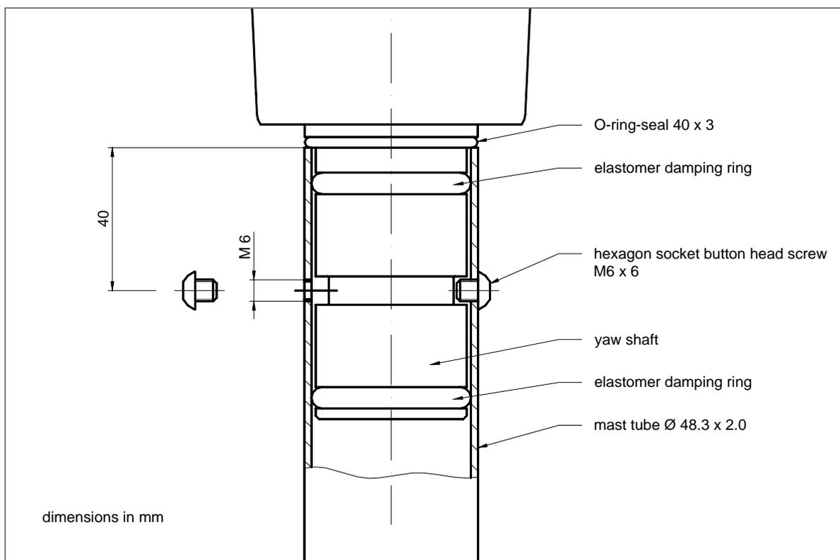
With this configuration the attached plastic bushing and the two socket cap screws M 6 x 8 (with the rubber rings on their head) are not needed. For easy assembling the two elastomer damping rings and the inside of the mast tube should be well lubricated with Vaseline. Now insert the yaw shaft into the tube and push it until the O-ring seal 40x3 seats solidly at the face side of the tube. Please take care not to damage the damping rings during feeding in.
