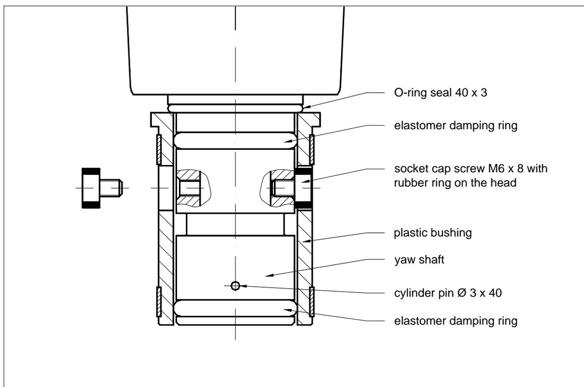
For mounting in mast tubes with inner diameter 55.0 mm the two adjusting rings have to be removed from the plastic bushing before the next working step can be carried out.
