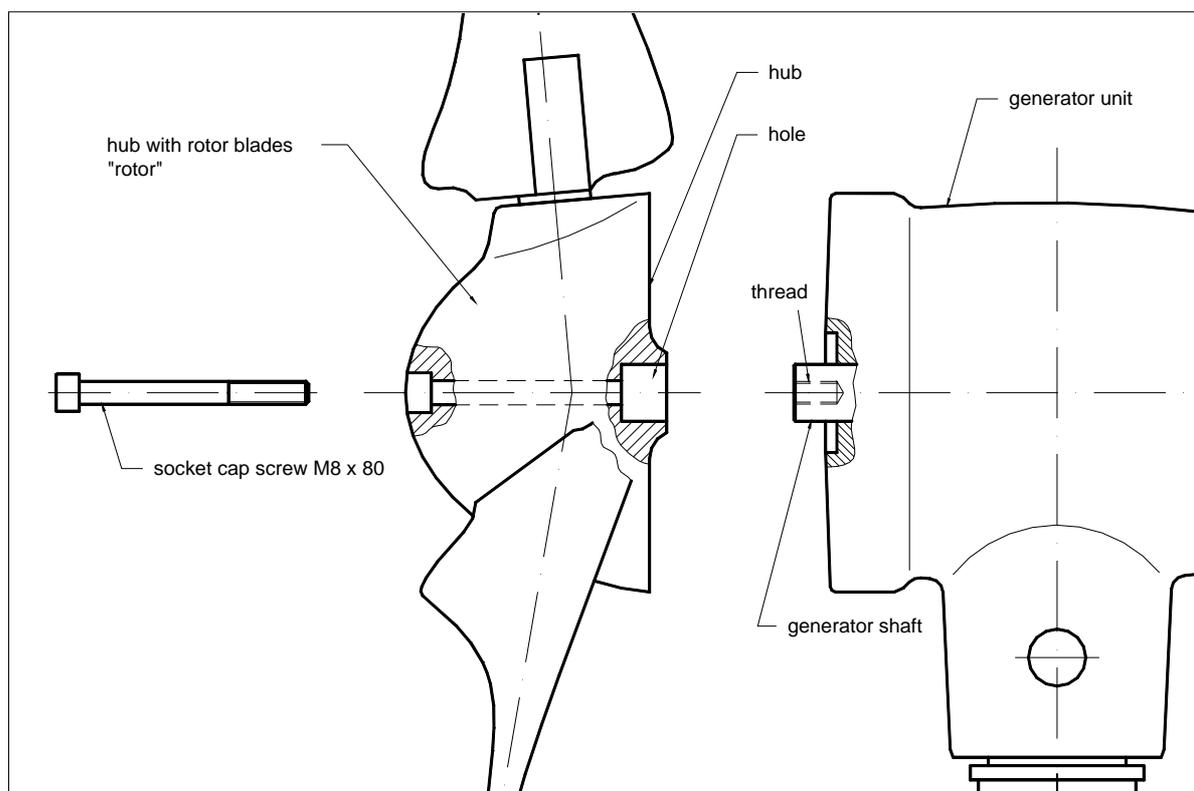
**NOTE:** To avoid damage inside the generator do not push the generator shaft into the generator housing (loss of warranty!).
